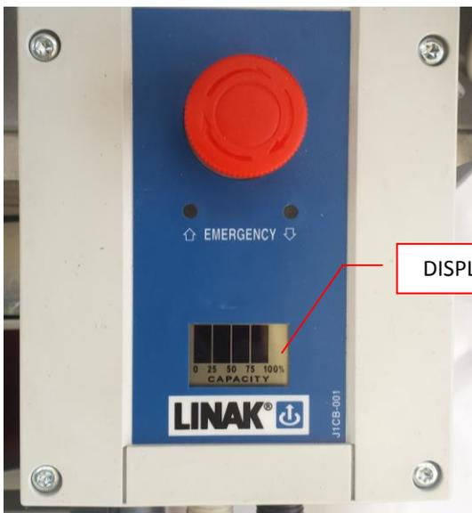
To check the status of charge of the battery is enough to check the lighting of the light switches placed on the display.
