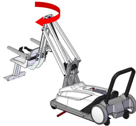
With the lowering button, proceed to the lowering until the immersion in water.
