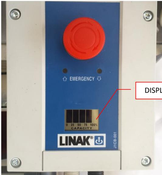
In normal operation the display shows the remaining battery power.
