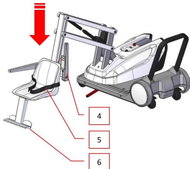
From the control panel, with the lifting button, move the seat to the maximum height.
