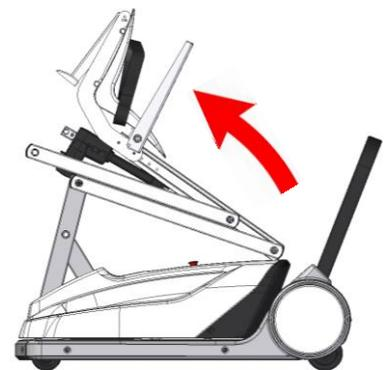
Align the mounting holes (A) of arms, frame and actuator.
