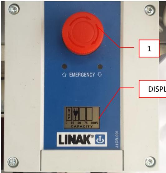
In case of pressing the emergency button (1) on the display the STOP warning appears and the machine stops.
