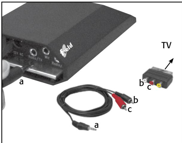
**2** Plug the transformer into a wall socket and into the power connection on the amplifier
