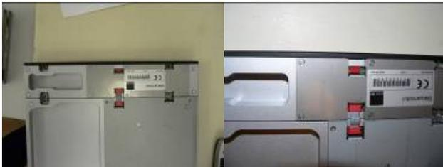
The red plugs are electrical contacts between the Braille display and the module. The ribbon-cable supplied with the module is inserted into this connector. Finally, the facing can then be screwed onto the module.
