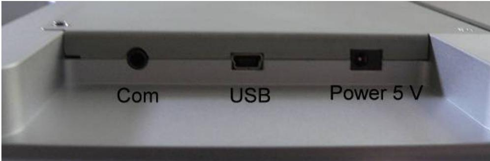
The communications channels/ports are located in the recess at the rear of the device on the right, approximately 2 cm deep. On the far left is the round socket for the serial port; in the middle the square socket for the USB port (mini-USB port) and on the far right the mains adapter socket (5 volt).
