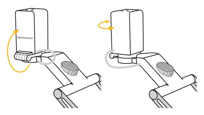
Using the round cross bar as the pivot, pull the camera head and LED light arm up and towards yourself until the LED lights are pointing down towards the table.
