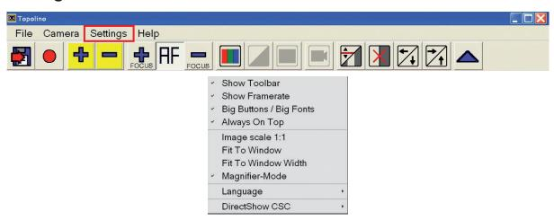
**Show Toolbar:** Use this option to turn the icon tool bar on and off. This toolbar is located right below the menu bar.
