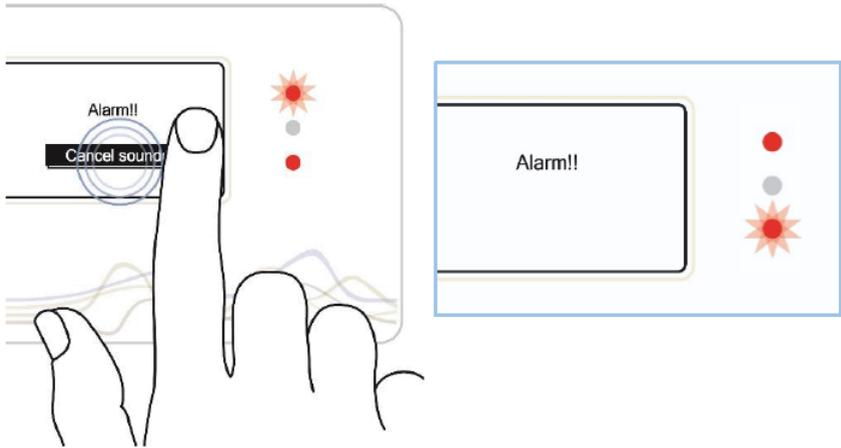
To turn off the alarm permanently, or reset the pump after fixing the cause of the alarm, simply switch the pump unit off and then on again.
