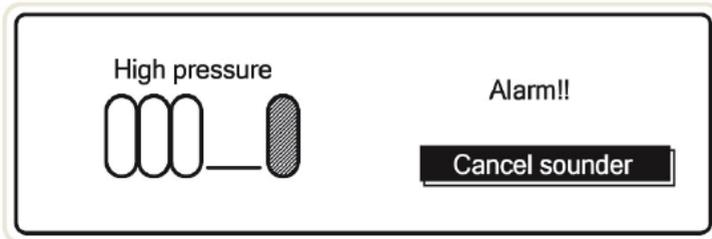
To resolve this issue, carefully push the CPR button and let out a small amount of air and then re attach the hose end. Reset the pump afterwards. Persistent high pressure alarms may indicate an internal fault. If it occurs mattress system use should cease. The pump should immediately be sent for servicing
