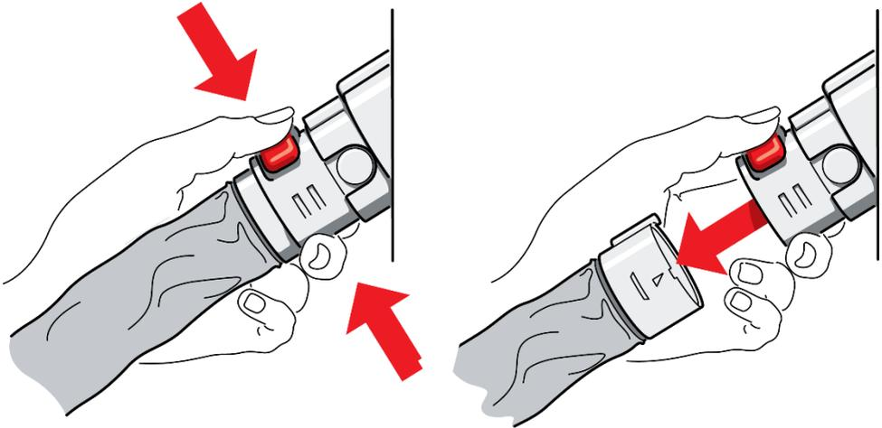
To deploy this emergency system, simply grip the CPR unit and push the RED BUTTON. The hose end closest to the mattress should spring out and the mattress will rapidly deflate.
