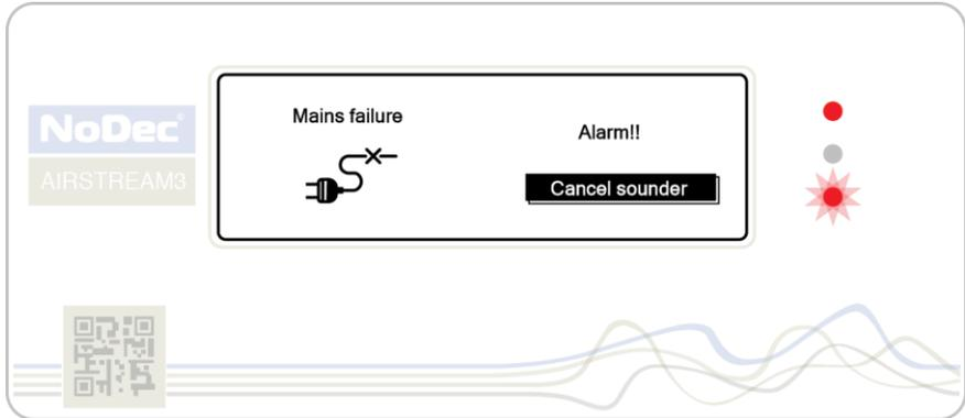
It is possible to resolve this alarm by simply plugging the power cable back into the mains, without the need to reset the control unit however this depends on the region.
