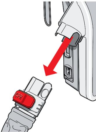
Simply push the buttons on the sides of the umbilical dock and the umbilical will disconnect. The mattress itself will remain inflated for several hours.
