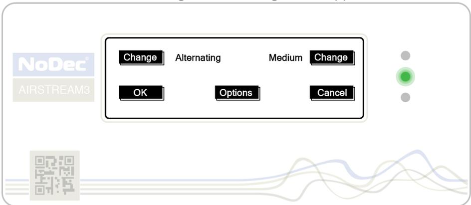
After 20 seconds of inactivity, the system will automatically lock out the display touch screen.
