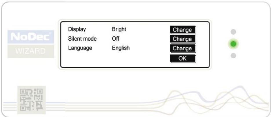
Here it is possible to 'Dim' the display and turn on 'Silent Mode', both of which may be useful during night hours in a hospital ward environment.
