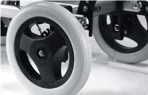
Ulike størrelser for drivhjulene (her 12") Various sizes for the back wheels (here: 12")
