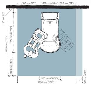
Blue area shows the minimum working area required for the staff to be able to use the mechanical aids in an ergonomic way from one side.
