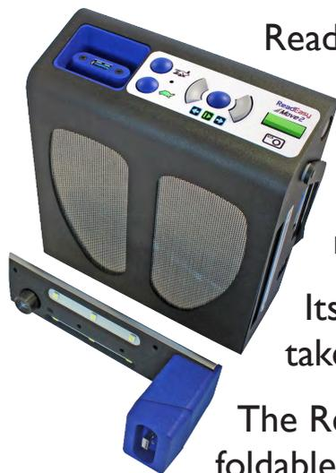
ReadEasy Move 2 features a unique magnetic quick release camera system. Simply placing the camera into its dock on the base unit automatically locates it into the correct position.
