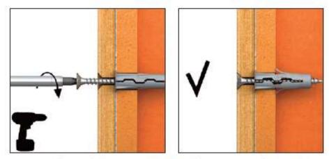
Insert screw of required diameter into plug, through fixture mounting plate & tighten.
