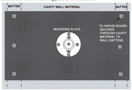
Additional strength may be achieved by using a suitable adhesive between the board and the cavity wall.
