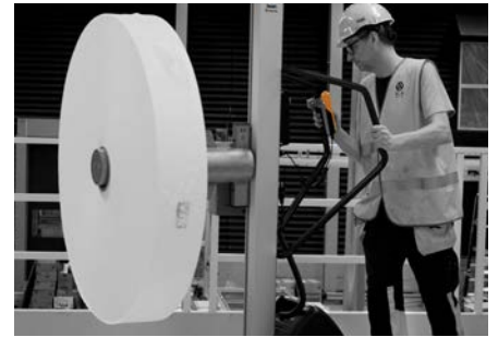
Lifting trolleys offer easy and ergonomic lifting, moving and tilting of goods such as rolls and drums, with full flexibility and mobility.
