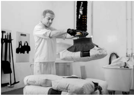
Vacuum lifters offers sustainable, safe and efficient handling of most types of goods up to 270kg.
