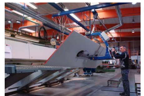
The sheet gripper is ideal for handling sheets of wood.. Add a tilting function and you can easily tilt loads of up to 250 kilos, up to 180 degrees.
