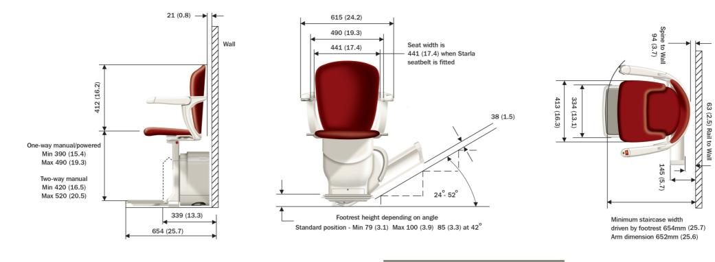
Measurements are in millimetres. Measurements in brackets are inches. All dimensions measured from the wall are nominal. The addition of a wide stringer or similar obstruction may affect the dimensions taken from this point. The colour representation of the chair shown here is for illustrative purposes only. Weight limit note: Upto 52° - 160kg (approx 25 stone)
