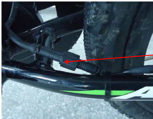
Water proof connector for speed detecting sensor
